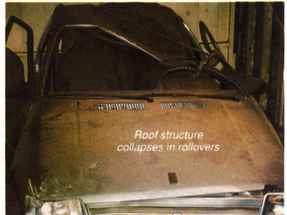
Further aggravating the roof integrity situation are designs that include too many holes, cutouts, notches, dimples, creases, and other discontinuities... plus a minimal number of widely spaced spotwelds, often poorly located along minimal flanges. Because of these needless design defects, the roof is structurally pre-disposed to buckle and collapse.
