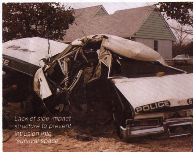
Lack of side impact structure to prevent intrusion into "survival space"
