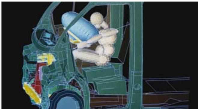
Left: Simulated and physical crash tests can ensure the cabin protects the driver in rollover accidents
